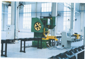
Semiautomatic CNC Punching Machine for Angles Model AP16A-8
