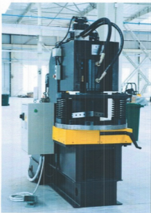
Hydraulic Notching Machine for Angles Model ACH200
